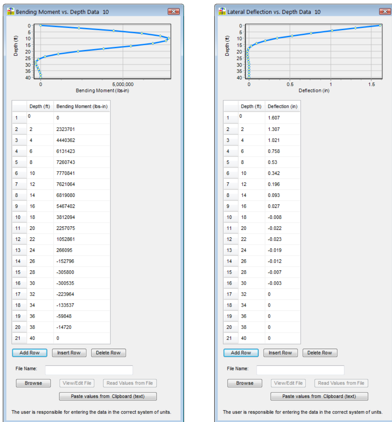
Figure 3-58 Dialogs for Input of Bending Moment and Lateral Deflection versus Depth from Load Testing.
